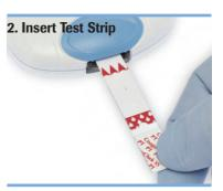
Slide the test strip into the test strip guide in the direction of the arrows until it stops.
