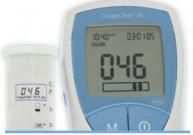
Confirm that the number displayed matches the number on the test strip container, then press M
