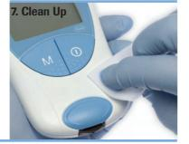
Place the used test strip and lancet in an approved container. Turn the meter off If the meter is dirty, wipe it clean with a CoaguWipe™ Bleach Towel.
