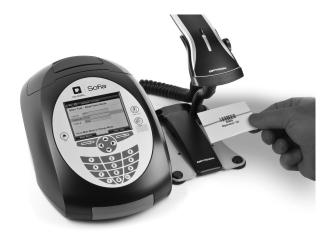
3. Input Patient ID or Order # using the barcode scanner or manually enter the data using the key pad.
