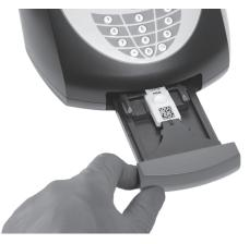
**8.** Sofia will start automatically and display the progress, as shown in the example below. The test results will be displayed on the screen in approximately 3 minutes. See Interpretation of Results section.
