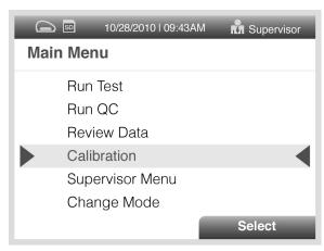
2. Following the prompts, insert the Calibration Cassette into Sofia and close the drawer. Sofia performs the calibration check automatically with no user input required.
