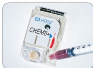
Step 1: Insert two or three drops of blood into the cartridge
