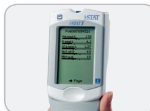
Step 3: View the results on the handheld screen within minutes
