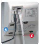
Plug the power supply (A) into the Cholestech LDX and the wall or power strip. Insert the end of the white printer cable (B), labeled "To Cholestech LDX," into the Analyzer.
