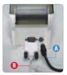
Plug the printer power supply A into the printer and the wall or power strip. Connect the end of the printer cable 3, labeled "To Printer," to the printer.
