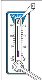
This is an example of unacceptable development of the QA Spot. The result should be considered invalid. Repeat the test using a new Q.E.D. device.
