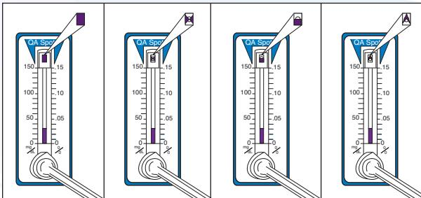
These are examples of acceptable development of the QA Spot. Read alcohol concentration from the end of the color bar. All of these devices read 30 mg/dL (0.03%).
