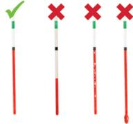
5. Inspect the capillary tube for proper filling. Make sure there are no gaps or bubbles, or any excess control on the outside of the capillary tube.
