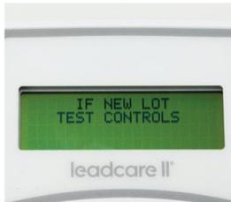
5. Calibration takes a few seconds. When calibration is complete, the screen briefly reads "CALIBRATION SUCCESSFUL". Then the screen reads "IF NEW LOT TEST CONTROLS", followed by the "PREPARE SAMPLE..." message.
