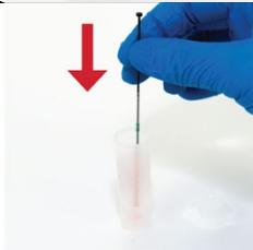
2. Place the full capillary tube in the treatment reagent. Insert a plunger into the top of the capillary tube and push down, ensuring to dispense the entire volume into the treatment reagent.
