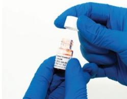
2. Swirl the control vial gently. Remove the cap from the control and place it *top down* on a clean laboratory wipe. Ensure the lot number on the control vial matches the sensor lot number you will be testing.
