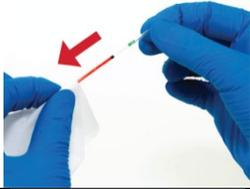
4. Use a downward motion to remove excess control from the outside of the tube with a clean wipe or gauze pad. Use caution not to absorb the control from the end of the capillary tube.
