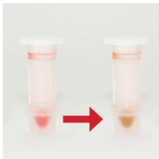
4. The test sample is ready when the mixture turns brown. Repeat sample collection and preparation for each sample to be tested.
