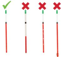
4. Inspect the capillary tube for proper filling. Make sure there are no gaps, air bubbles, or any excess blood on the outside of the capillary tube.
