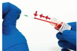
3. Holding the capillary tube almost horizontally with the green band on top, fill it to the 50  $\mu\text{L}$  **black line**. Replace the cap on the control vial.
