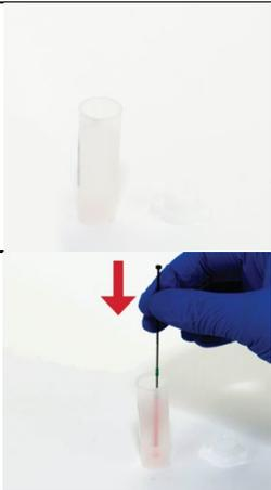
6. Remove the cap from a vial of treatment reagent and place it *top down* on a clean surface. Do NOT allow the inside of the cap to touch anything. This could cause inaccurate test results.
