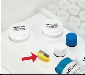
2. Locate the calibration button in the test kit. Remove the calibration button from the test kit package.
