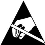
This symbol indicates the potential for electrostatic discharge. Static electricity can damage or destroy the internal components of devices. It can be generated by scuffing shoes on a carpet or brushing some other materials such as fabrics. When running the analyzer, discharge static electricity by touching a metal object (such as the outside of a computer) in your work area.
