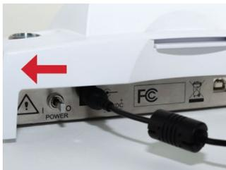
1. Turn on the analyzer. The analyzer is ready when the “Prepare Sample” message appears.
