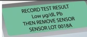
**NOTE:** The analyzer displays “Low” when it detects a blood lead level below 3.3 µg/dL. “Low” results should be recorded as “<3.3 µg/dL”. It is not uncommon to obtain patient results that read “Low”.
