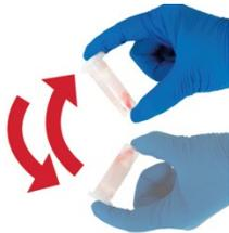
8. Replace the tube cap. Invert the tube 8 to 10 times to mix the sample completely. The mixture will remain red.
