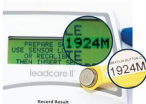
6. Make sure the number of the button matches the display. The LeadCare II Blood Lead Analyzer is now ready for testing.
