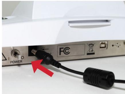
**Figure 1-3 Plug in DC Connector/AC Adapter**
