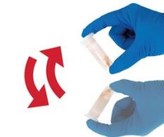
3. Replace the tube cap. Invert the tube 8 to 10 times to mix the sample completely.
