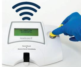
4. Hold the calibration button to the button reader until you hear the beep. The button must touch both the center contact and metal side of the button reader.
