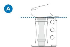
Double-check to make sure top of Swab is flat and even with top of Key.
