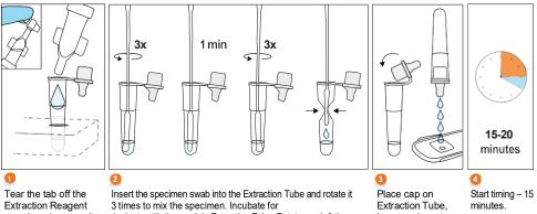
Extraction Reagent capsule and squeeze it to dispense all of the solution into the Extraction Tube.
