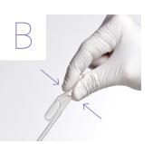
Squeeze the **upper bulb** of the provided pipette and submerge the tip to the **bottom** of the sample tube.
