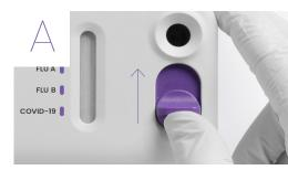
Slide the switch upwards in a firm, swift motion to close the sample port to start the test. **Do not move test** while running. Note: Make sure the switch is pushed all the way up.
