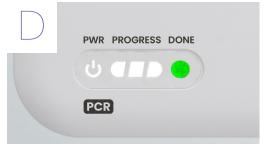
green light to appear indicating the test is finished running.
