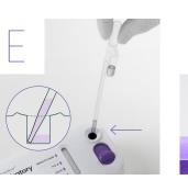
Place the tip at the **bottom** of the sample port and then squeeze the upper **bulb** of the pipette to release all of the sample.
