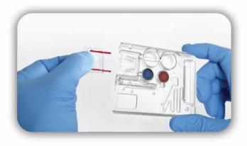
Insert sample into cartridge
