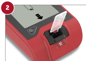
2 Place the microcuvette into the analyzer.
