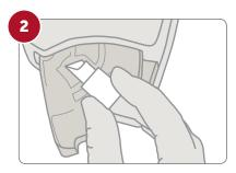
Place the microcuvette into the analyzer.
