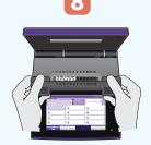
Lower the Reaction Tubes into Solana.
