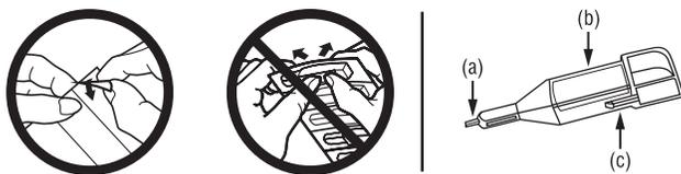
Discard the plastic capillary holder if any of the following are missing from the holder: (a) glass capillary, (b) absorbent pad, (c) latching mechanism.
