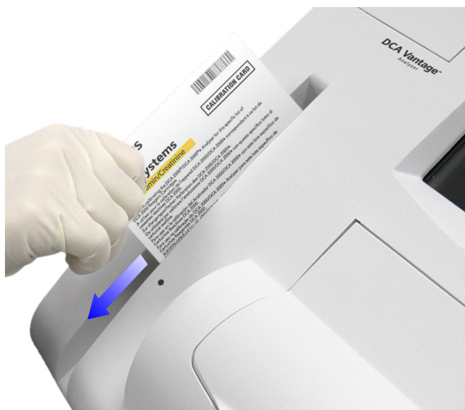
Figure 26 Scanning the Microalbumin/Creatinine calibration card
