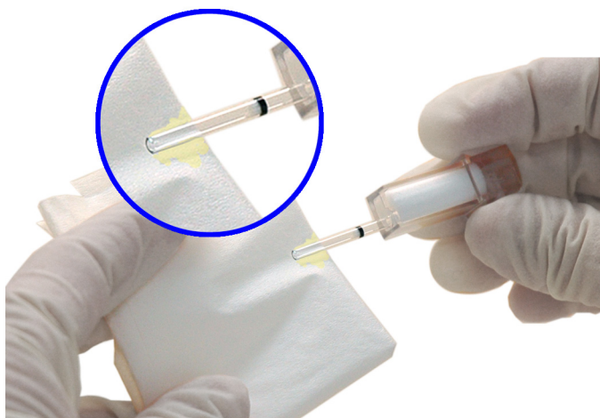
Figure 19 Wiping the Outside of the Glass Capillary Tube
