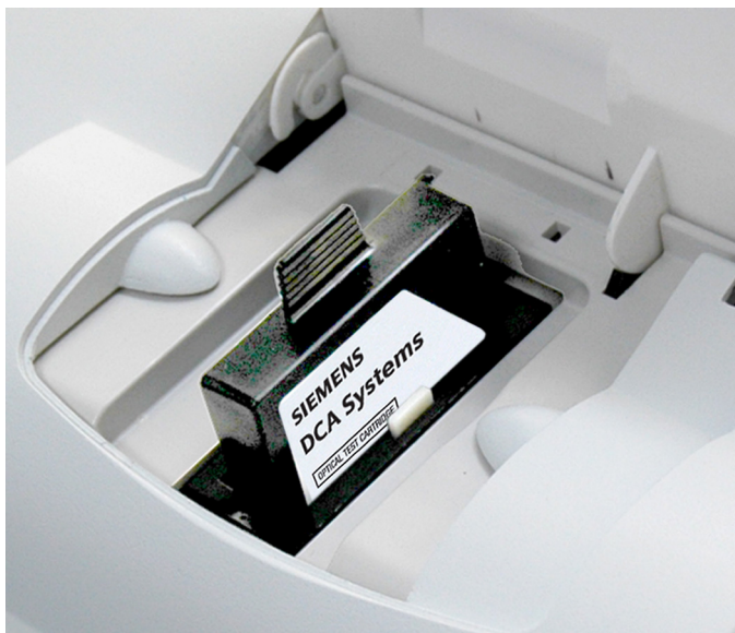
Figure 39 Inserting the Optical Test Cartridge into Compartment
