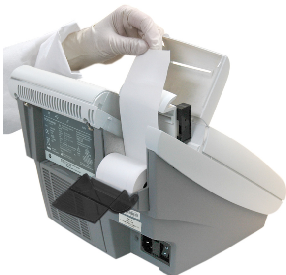
Figure 41 Inserting Paper into the Printer
