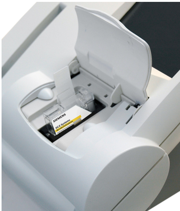
Figure 22 Inserting Reagent Cartridge into System
