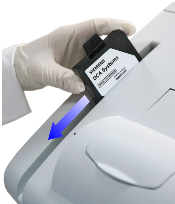
Figure 38 Scanning the Optical Test Cartridge
